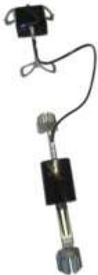
The KNEEMAP®, based on inertial power plant technology (accelerometers and gyrometers), is composed of mechanical and electronic elements, all controlled by a tablet. The KNEEMAP® provides a true mapping of all knee laxities to anticipate and adapt the future surgical gesture and evaluate it objectively.
